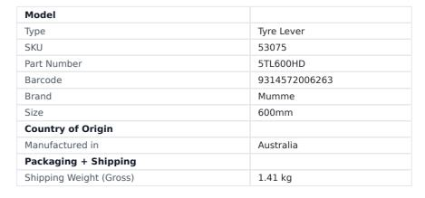
Stronger lever removes/fits tyres for commercial vehicles, agricultural and construction machinery
