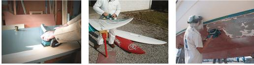
Similar to the CE23N model, but with an adjustable curved base for concave, convex and flat surfaces. Specially usefull for working in shipyards, where resins with fiberglass, carbon fibre and kevlar are used. Also for stripping layers of gel coat and paint. Equipped with dust collection nozzle.
