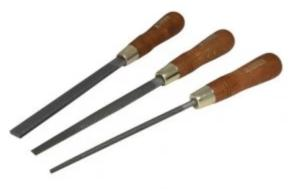
Rasp are suitable for shaping wood, plywood, panels, plastic and other soft materials. Blades are made of tool steel, heat treated to 49 HRc. Ergonomic handle is made of quality hard wood. Rasp teeth are suitably situated on the blade, so that the removal of material is steady and even.
