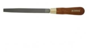
Rasp are suitable for shaping wood, plywood, panels, plastic and other soft materials. Blades are made of tool steel, heat treated to 49 HRc. Ergonomic handle is made of quality hard wood. Rasp teeth are suitably situated on the blade, so that the removal of material is steady and even.
