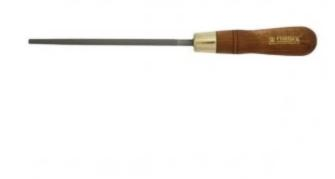
Rasp are suitable for shaping wood, plywood, panels, plastic and other soft materials. Blades are made of tool steel, heat treated to 49 HRc. Ergonomic handle is made of quality hard wood. Rasp teeth are suitably situated on the blade, so that the removal of material is steady and even.
