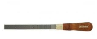
Rasp are suitable for shaping wood, plywood, panels, plastic and other soft materials. Blades are made of tool steel, heat treated to 49 HRc. Ergonomic handle is made of quality hard wood. Rasp teeth are suitably situated on the blade, so that the removal of material is steady and even.
