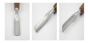
PROFI carving chisels are hand-made tools of the highest quality, designed especially for professional carvers. Blades are made from chrome-silicon alloy steel and heat treated for hardness of 59 ± 1 HRc. All blades are hand polished. The edges are sharpened and lapped with abrasive paste and arkansas stone. Handles have an octagonal barrel shape and are made of beach wood. The surface is stained and waxed.
