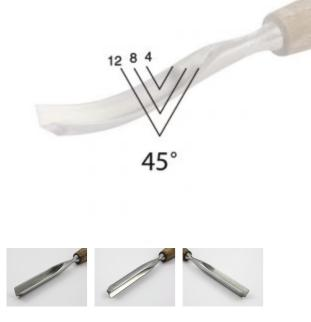
PROFI carving chisels are hand-made tools of the highest quality, designed especially for professional carvers. Blades are made from chrome-silicon alloy steel and heat treated for hardness of 59 ± 1 HRc. All blades are hand polished. The edges are sharpened and lapped with abrasive paste and arkansas stone. Handles have an octagonal barrel shape and are made of beach wood. The surface is stained and waxed.
