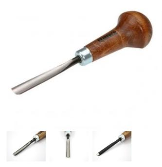
Graving chisels PROFI are handmade tools of the highest quality, designed especially for proffessional carvers. Blades are made of Chrome-Vanadium tool steel and heat treated to the hardness of 61-62 HRc. The edges are sharpened and lapped with abrasive paste and arkansas stone.
