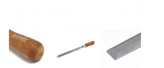
Paring chisel blade is made from highly alloyed Cr-Mn steel and heat treated up to 59 HRc. Ergonomic handle is made of hornbeam wood and is equipped with brass ferrule. Paring chisels are used primarily for carefully shaving off thin amounts of wood when fitting joints. The long length gives maximum control. These tools are always pushed by hand, they are never malleted.
