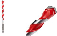
The Milwaukee® Hammer Drill Bits have been designed with a 2 cutter carbide tip to allow for drilling into concrete, brick, block and soft material for electrical installations, lighting fixtures and holders. Our Hammer Drill Bits also features a red flute for easy identification along with a wide flute design to remove dust faster, while also reducing heat build-up, resulting in more holes per charge. Available individual sizes range from 3mm up to 12mm.
