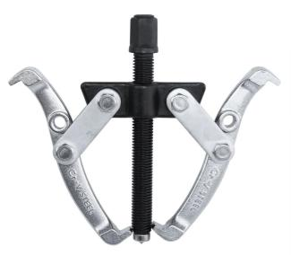
Available in 3 sizes: 75mm, 100mm & 200mm Easily remove gears, pulleys, bearings, sprockets and flywheels from shaft without damage Inside & outside reversible hooked jaws for external or internal pulling flexibility Twin hole reversible arms Centre screw with centre screw Chrome Vanadium Steel (Cr-V) for high strength and durability
