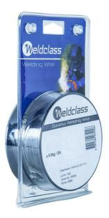
Gasless (self-shielded) 'MIG' Welding Wire in 0.9kg (100mm) mini-spools for small welding jobs and use in spool-guns. Weldclass mini spools are E71T-11 grade which is suitable for multi-pass welding - unlike many other mini-spools on the market that are E71T-GS grade & suitable for single-pass welding only. **Features:-**
