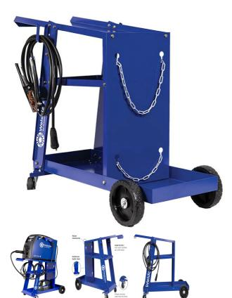
Robust welding trolley - the ideal platform for your portable welder or plasma cutter. **Now available with 7year warranty**. Outrigger caster wheel design for greater stability. Large upper tray with open-front design accommodates small or large machine, including most portable MIG welders up to 250A. Overall Size (mm): 1,000L x 720H x 420W (including axle). Size of top tray (mm): 700L x 275W. Includes 2 gas bottle chains and 2 lead/cable hanger hooks.
