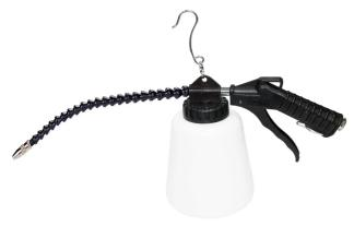
PE tank and tube with adjustable spray/jet nozzle Flexible tube Lance with adjustable nozzle with cone Capacity: 1 Litre
