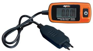
Available in 2 size options: Standard-blade or Mini-blabe Tests circuit current up to 30Amps Design allows for easy connection into fuse Sockets Maintains fuse protection while connected Resolution .1A (100 milliamps), accuracy +2
