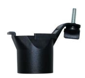
Replacement dust port adapter for HL 850 Planer, enabling connection to chip collection bag or to CT suction hose. The 36 mm diameter suction hose is recommended for effective chip extraction with a high volume chip producing tool such as the HL 850 Planer.
