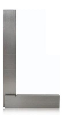
Squareness to BS939 standards. Spring steel blades hardened to 52-55HRC. Use of tapered self locking rivets ensures perfect rigidity. Both blade and stock are precisely ground to ensure straightness and parallelism.
