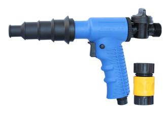
Multipurpose cleaning gun uses a combination of high pressure compressed air and water to quickly clean dirt, scale etc from the cooling system Multi-step nozzle suits most radiator and heater hose sizes
