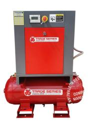
1100L/pm @ 116PSI - great workshop screw compressor. 8 Bar / 116PSI. Get as a base, tank mount or full feature with screw, dryer and tank as one.
